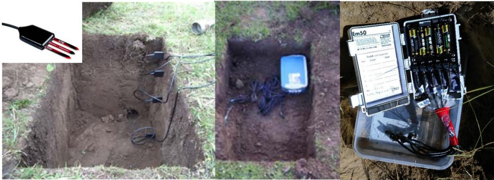
Figure 2. An example of instruments configured for each SMST monitoring site.
